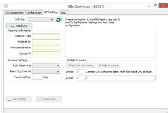
The configuration tool should automatically detect the correct COM (Serial) port number. If you have more than one serial port, you may need to manually adjust the 'COM Port' setting to match the port that the GPS is connected to.
