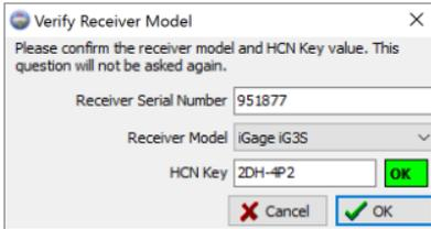
Use the drop down 'Receiver Model' to change the receiver type. If the HCN Key has been lost, it is written on a white sticker inside the battery compartment. You cannot edit the 'Receiver Serial Number'.
