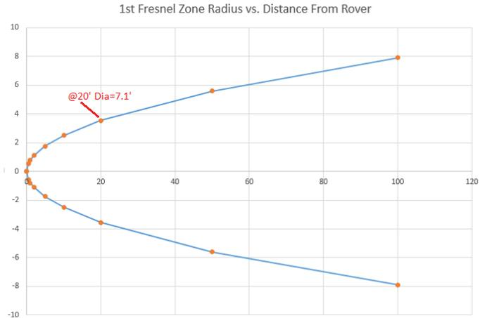
1 foot above your GNSS antenna, the beam width is 1.6' in diameter. 20 feet above the rover antenna (perhaps the midpoint of tree canopy), the 1<sup>st</sup> Fresnel beam diameter is 7 feet! A clearing in the treetops 100' above your antenna needs to be 16' in diameter.
