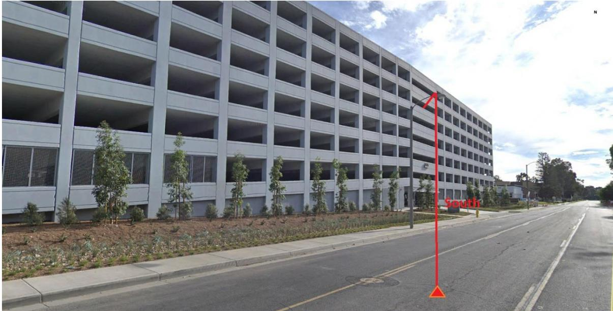
This is a **bad** location because the structure completely blocks the antenna's view to the South and East:
