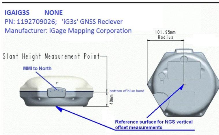
Have the MMI (Man-Machine-Interface) rotated to the north.
