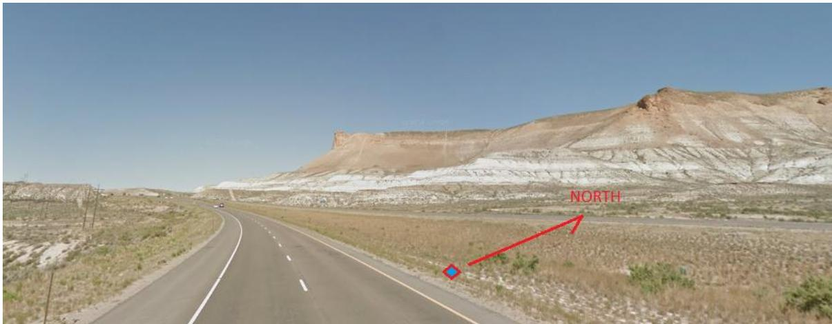
It has fantastic views in all directions, unfortunately a semi-truck drives by every 30-seconds and completely obscures a receiver's view of the southern sky. This forces the receiver (and OPUS) to lose lock. This is a **BAD** location and will greatly increase the RMS error estimates and drop the percentage of observations used.
