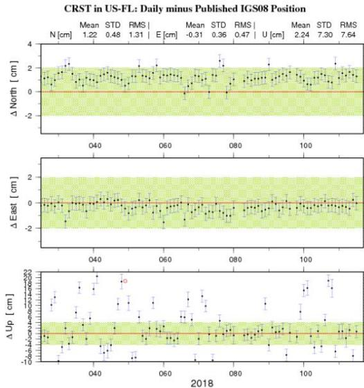
Again, this site should never be used in an OPUS solution. Both of these stations and all the others like them are unsuitable for any processing use.
