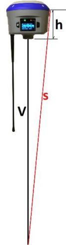
Slant reduction error is a very common source of bad instrument height. If you don't explicitly understand the slant measurement process, you absolutely should be using a fixed height pole.
