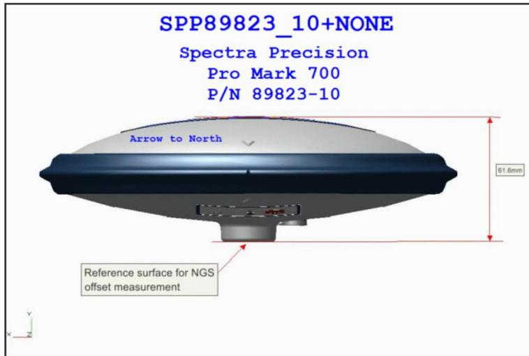
Some antennas like the ProMark 700 above have a North Arrow fiduciary mark which is rotated so the mark is to the north. Some antennas like the iG3s:
